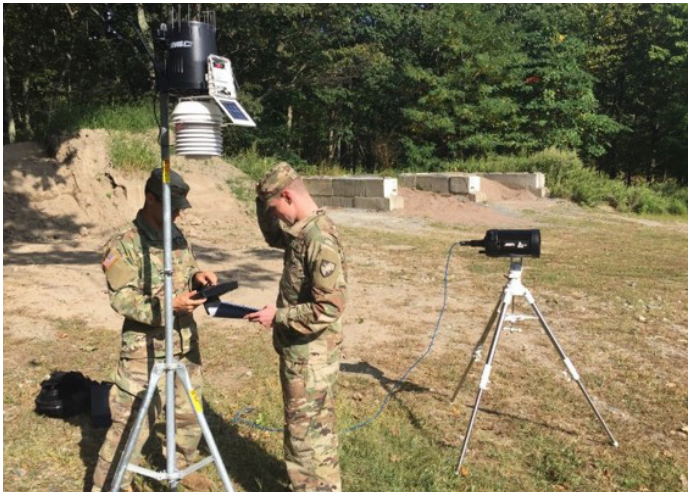
Cadets establishing a monitoring station on Range 4A, or the Outdoor High Energy Laser Laboratory (O-HELL), at West Point, NY to study the effects that various weather conditions have on optical turbulence. This work will enable commanders to more effectively employ directed energy systems on the battlefield.
