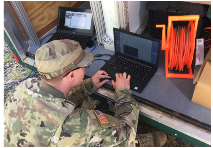
Cadets establishing a monitoring station on Range 4A, or the Outdoor High Energy Laser Laboratory (O-HELL), at West Point, NY to study the effects that various weather conditions have on optical turbulence. This work will enable commanders to more effectively employ directed energy systems on the battlefield.
